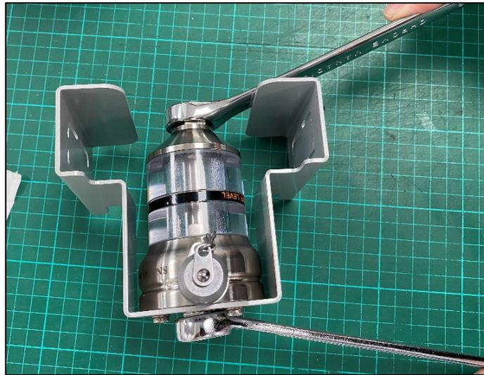
3. **Hold the water trap over a sink or receptacle and allow the water/contaminant to flow out.**
